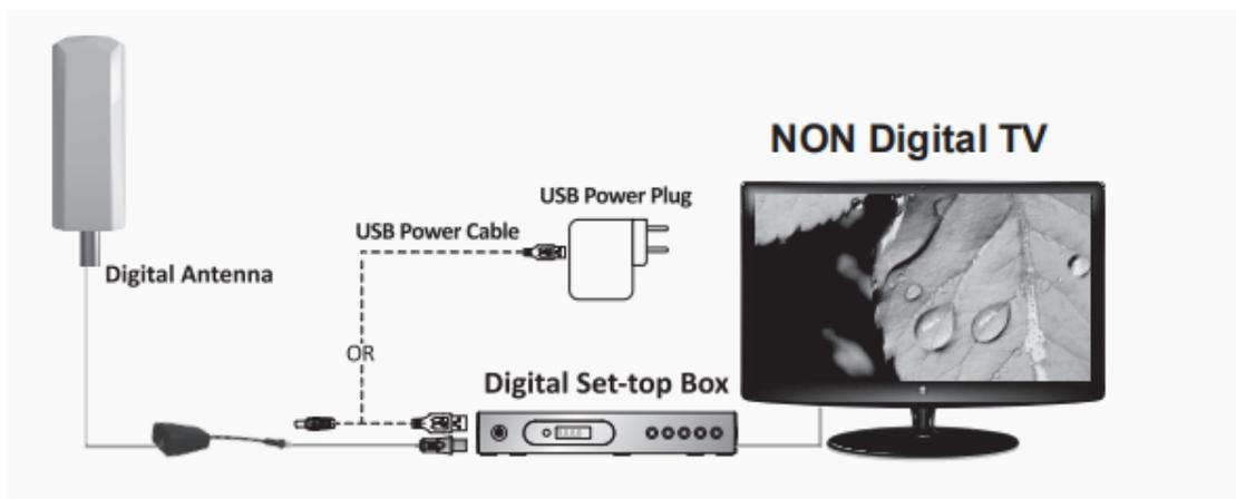
Connect the signal cable from the antenna to the signal input jack of the power supply, connect the power supply output jack to the digital receiver, plug the power adaptor with the power supply and connect to power socket, and finally join the TV and the digital receiver.
