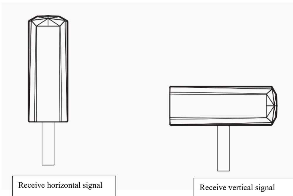
Adjust the antenna direction until you get the good signal for clear picture.
