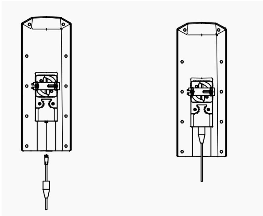
Connect the signal cable to the signal output jack of the antenna and then fix the waterproof cap covering the connections to avoid water filtration.
