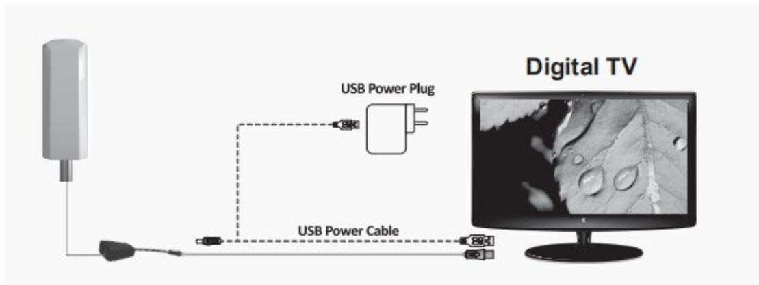
Connect the signal cable from the antenna to the signal input Jack of the power supply, connect the power supply output jack to the TV, plug the power adaptor with the power supply and connect to power socket.
