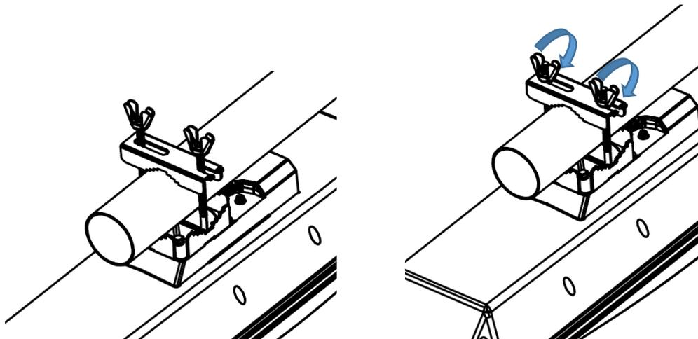
Place U-bolt through the mast, adjust the antenna bracket and fasten screws.
